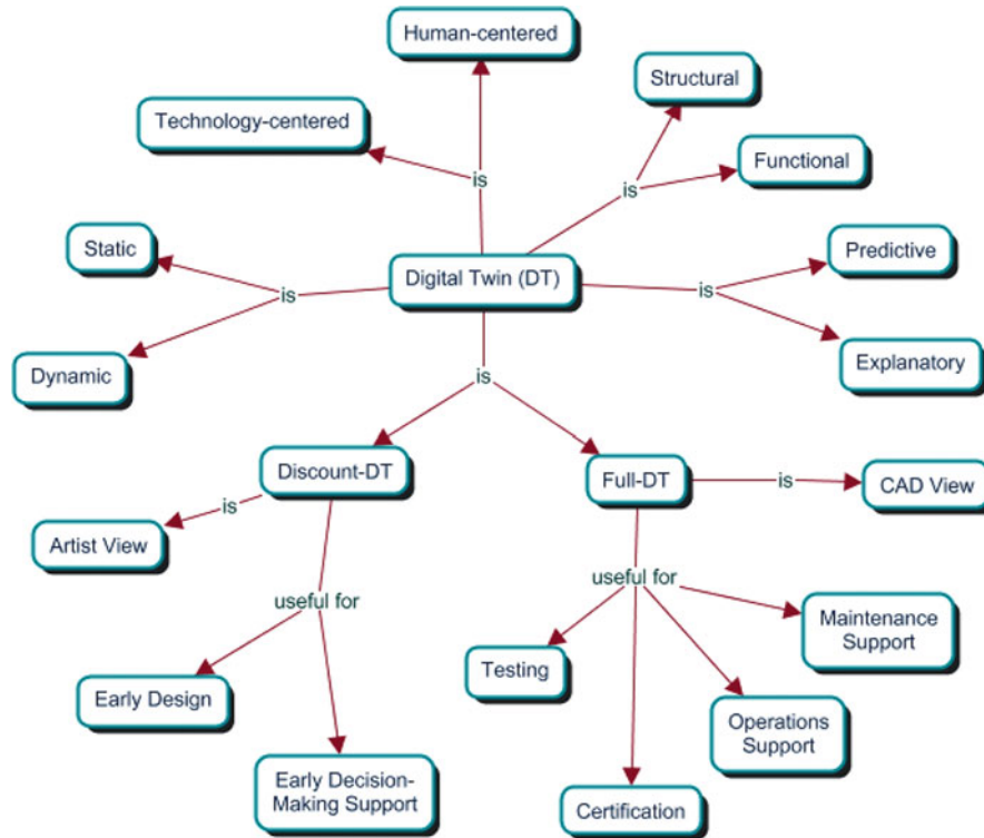
Fig. 2 Digital twin definitions and properties
